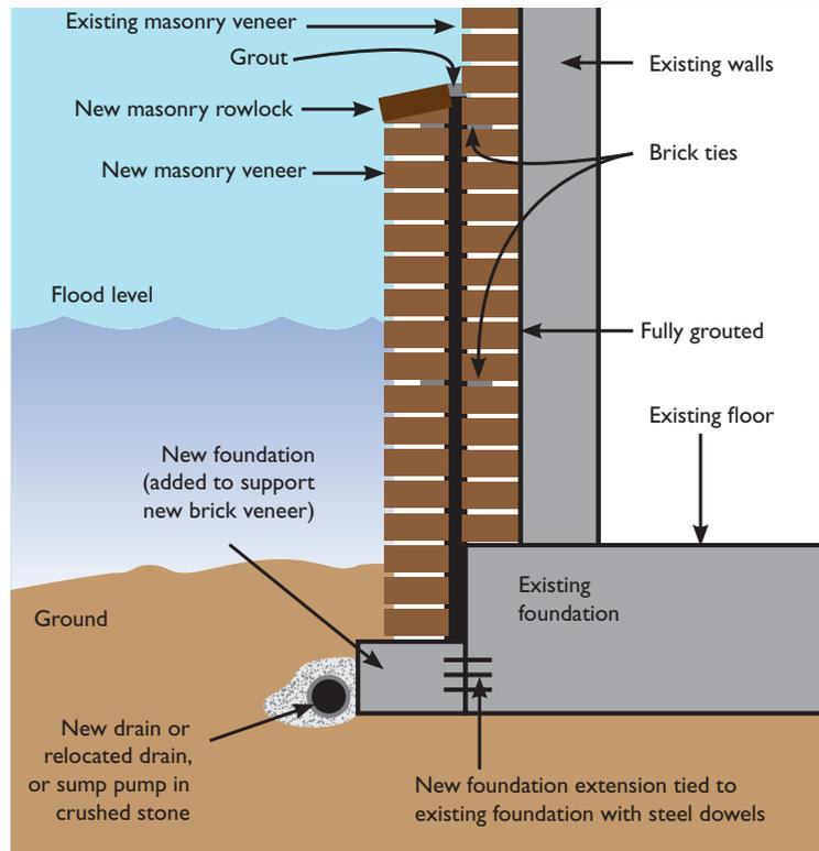
(Above) "A way to seal an existing brick-faced wall is to add an additional layer of brick with a seal in between. Please note that weep holes (drainage) and wick drains are moved up to prevent moisture from getting inside the walls." Images and descriptions provided by FEMA P-312, Homeowner's Guide to Retrofitting 3rd Edition (2014)
