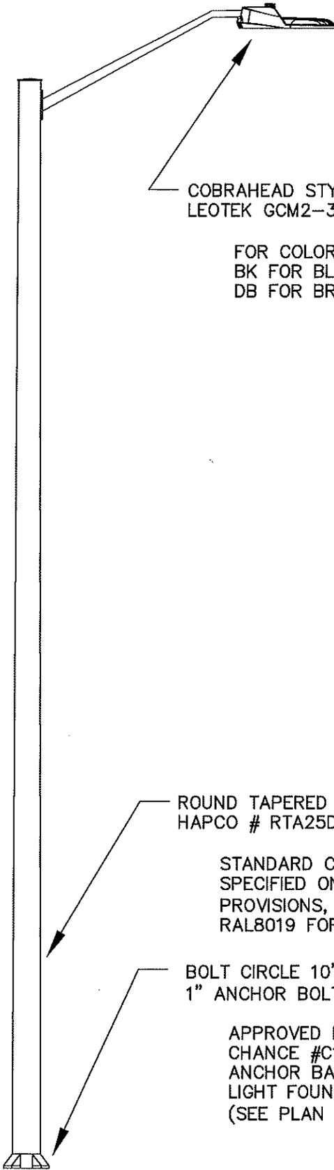
COBRAHEAD STYLE LED LUMINAIRE - 100 WATT EQUIVALENT
